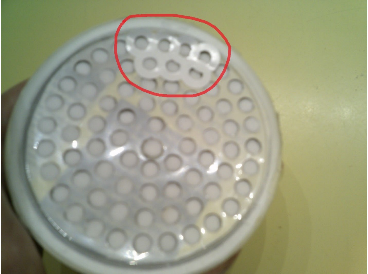
(Above) Seven reinforcing rings block access to the junctions between filter and cardboard matrix.
