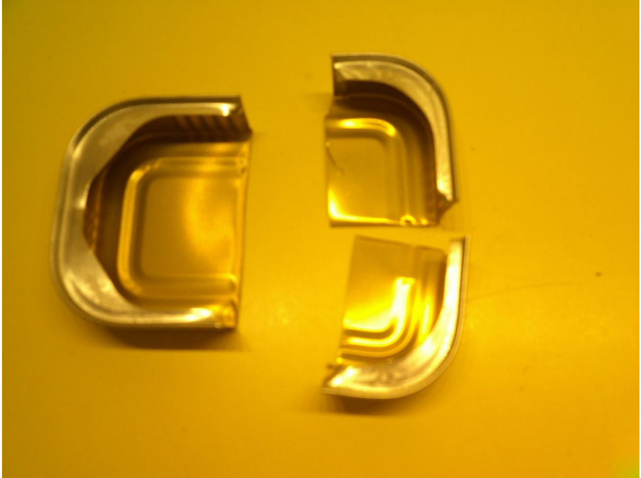
(Above) Cut the sardine tin into quarters.
